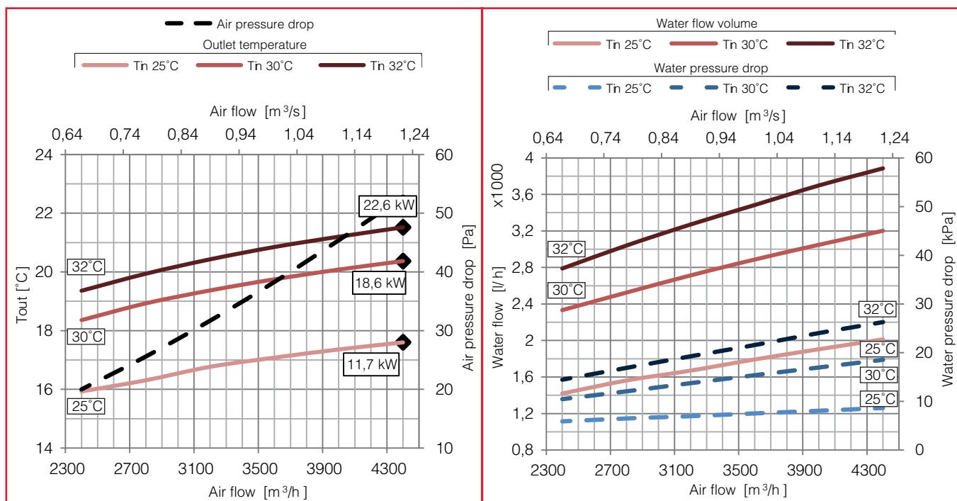
Heating water coil (45°C/35°C)
