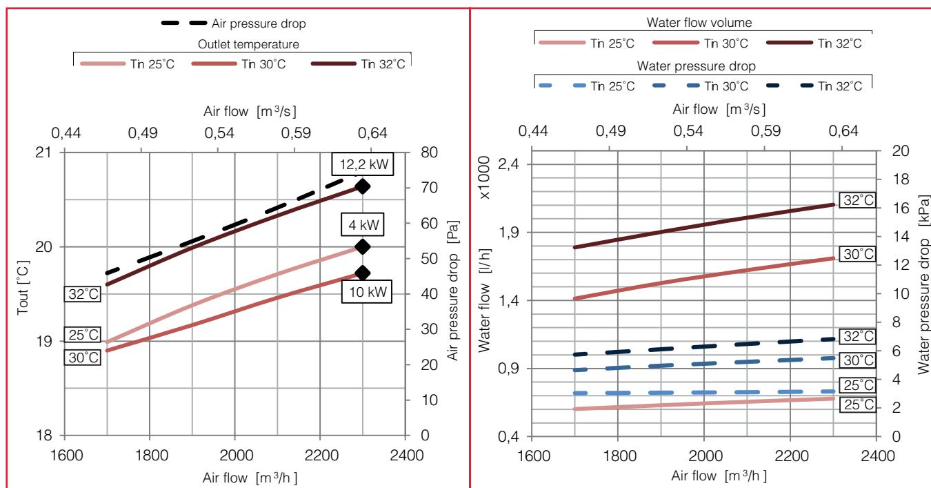
Heating water coil (45°C/35°C)
