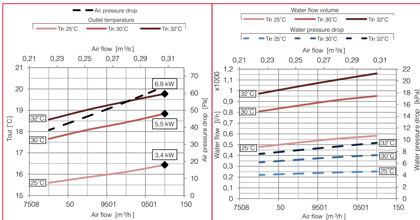
Heating water coil (45°C/35°C)
