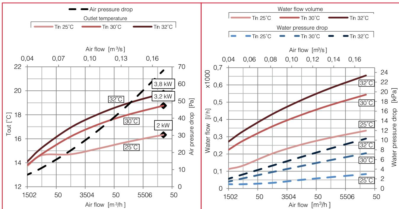
Heating water coil (45°C/35°C)
